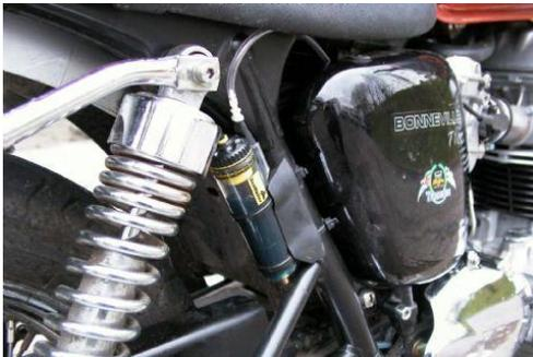
The delivery tubing can be routed along the swingarm using conduit and glue or self adhesive cable clips and the dispenser can be secured on the rear spindle using a Dispenser plate & Clip. For further information see our easy step installation guide - [Dispenser Assemblies, General](#). The nib should feed the rear sprocket between the 6 & 7 o'clock positions, with the cut face outwards.
